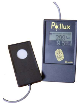
Digital radiometer/luxmeter simultaneously displaying illuminance and (UV-A) irradiance figures.
